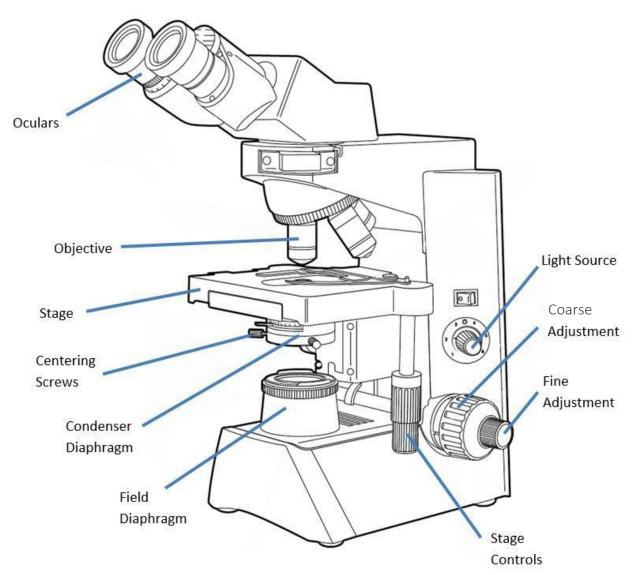
Oculars, Objective, Stage, Centering screws, Condenser diaphragm, Field diaphragm, Light source, Coarse adjustment, Fine adjustment, Stage controls
